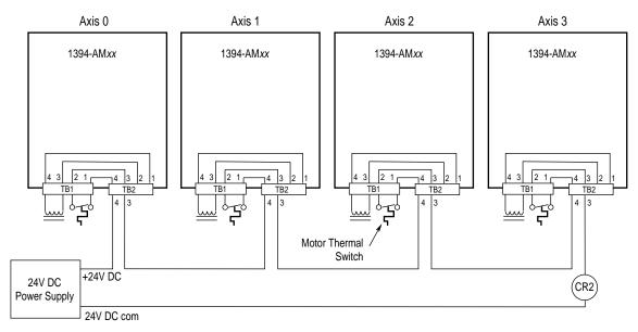
Note: 120V AC (50 or 60 Hz) power may be used in place of a 24V DC power supply for motor thermal switch circuits.
