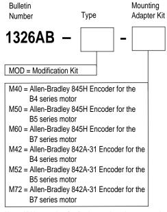
Note: All kits contain a feedback mounting adapter, mounting hardware, and a coupling. The kit does not contain a feedback device.
