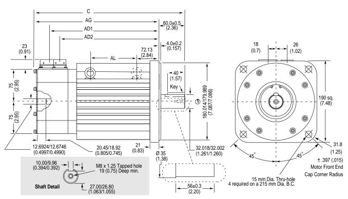
Figure A.22 1326AS-B6 Series Servo Motor
