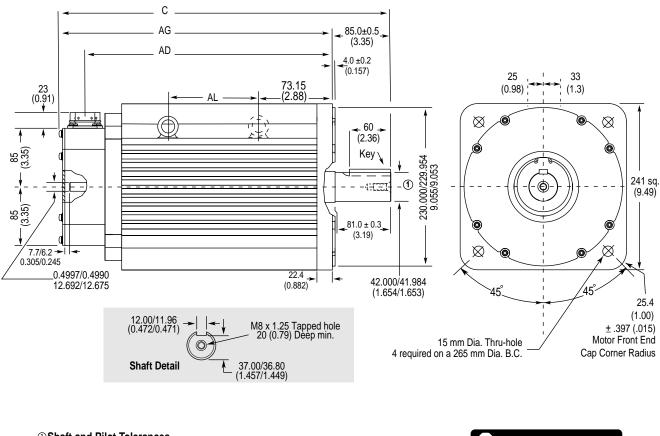
Figure A.23 1326AS-B8 Series Servo Motor
