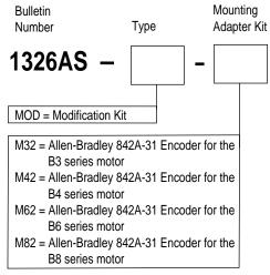
Note: All kits contain a feedback mounting adapter, mounting hardware, and a coupling. The kit does not contain a feedback device.
