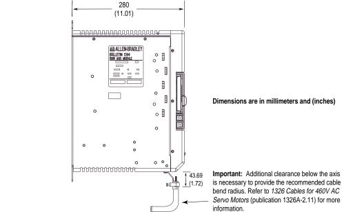
Figure A.8 1394C-AM50-IH and -AM75-IH Axis Module Side View
