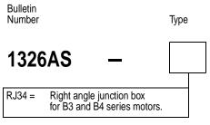
Note: The motor comes standard with IP65 plug style connectors mounted radially to the motor. This kit allows the connectors to be brought out axially to the motor without further wiring. Kit includes a motor junction box and mounting hardware.
