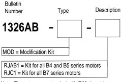
Note: The motor comes standard with IP65 plug style connectors mounted radially to the motor. This kit allows the connectors to be brought out axially to the motor without further wiring. Kit includes a motor junction box and mounting hardware.
