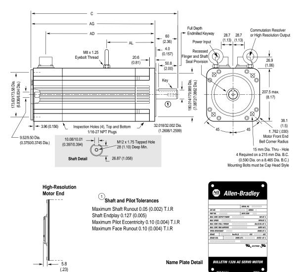
Figure A.19 1326AB-B7 Torque Plus Series (Resolver and High Resolution Feedback)
