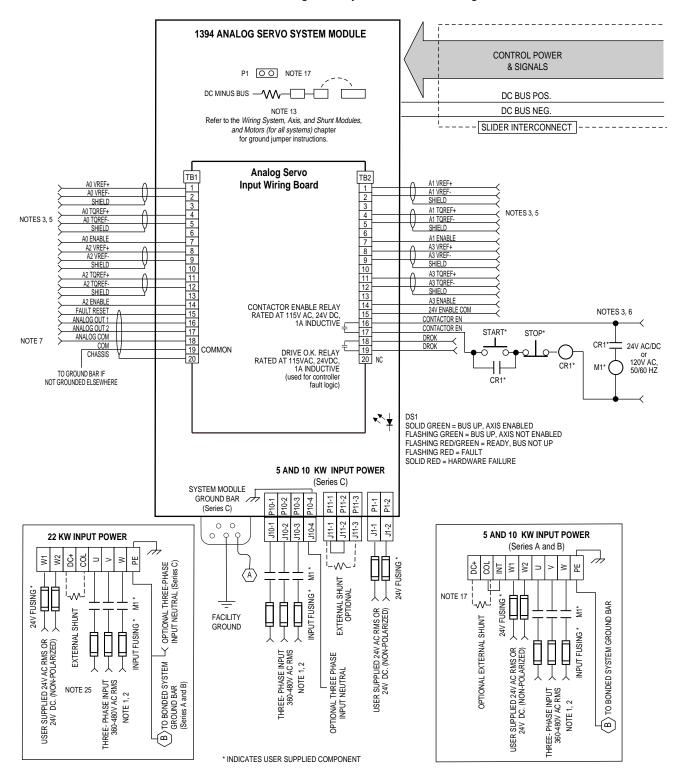
Figure B.6 Analog Servo System Interconnect Diagram
