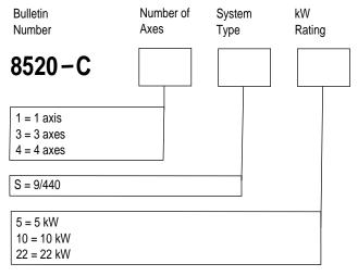
Note: 8520-C (Series C) system modules include Smart Power, improved terminations, and EMI filtering. Refer to 9/Series Integration and Maintenance Manual (publication 8520-6.2) for more information.
