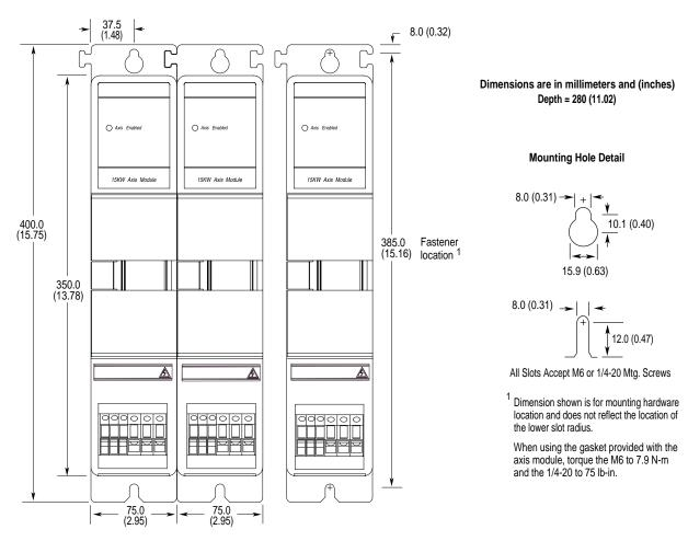
Figure A.6 1394*x*-AM50, -AM50-IH, -AM75, and -AM75-IH Axis Module Front View
