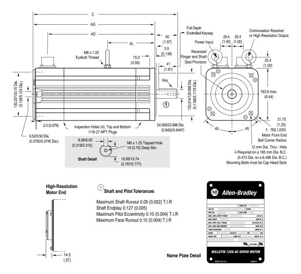
Figure A.18 1326AB-B5 Torque Plus Series (Resolver and High Resolution Feedback)
