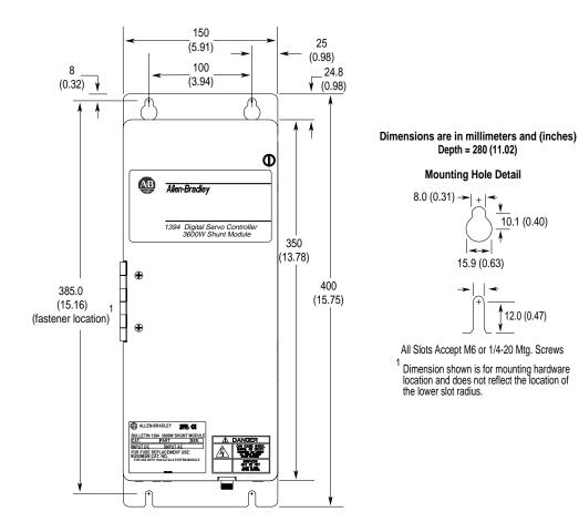
Figure A.15 1394-SR-36A and -36AF Front View Dimensions
