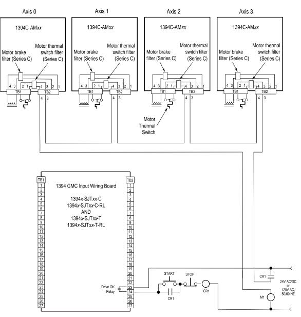
The example below shows 1394 (Series C) axis modules wired for thermal fault monitoring. Depending on how the 1394 GMC system is configured, the fault can be used to disable one or all of the four axis modules.
