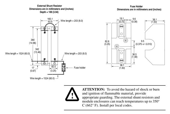
Figure A.13 1394-SR-9A and -9AF Front View Dimensions
